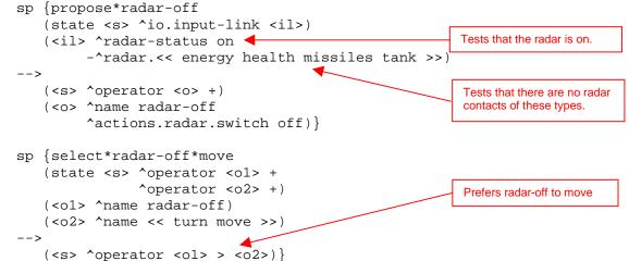
A different approach is to turn off the radar as part of the move operator. Turning the radar off can happen in parallel with moving and turning. It is implemented as an additional action of those operators.
